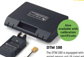
The DTM 100 is equipped with a patented sensor unit (K-type) with sensor wires made of chromel and alumel. It provides exact temperatures of even finest soldering tips.
