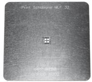
Dip stencil, 20 x 20 mm, 150 µm
