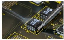
Efficient solder fume extration directly at the solder joint
