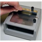
Flux application in a dip stencil
