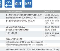
Standard accessories included Test lead (TL-61), Instruction manual The value in ( ) at DCV and ACV is input resistance.
